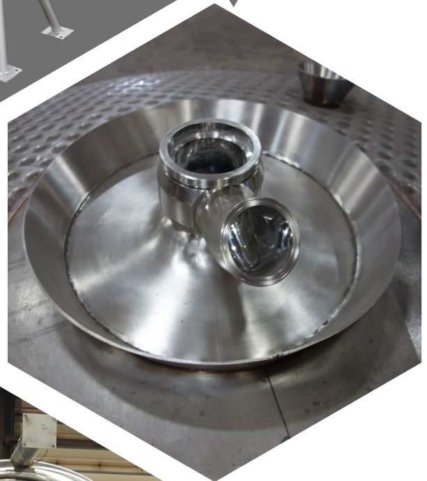
Dimple jacketed ASME Vessel Bottom ▼
