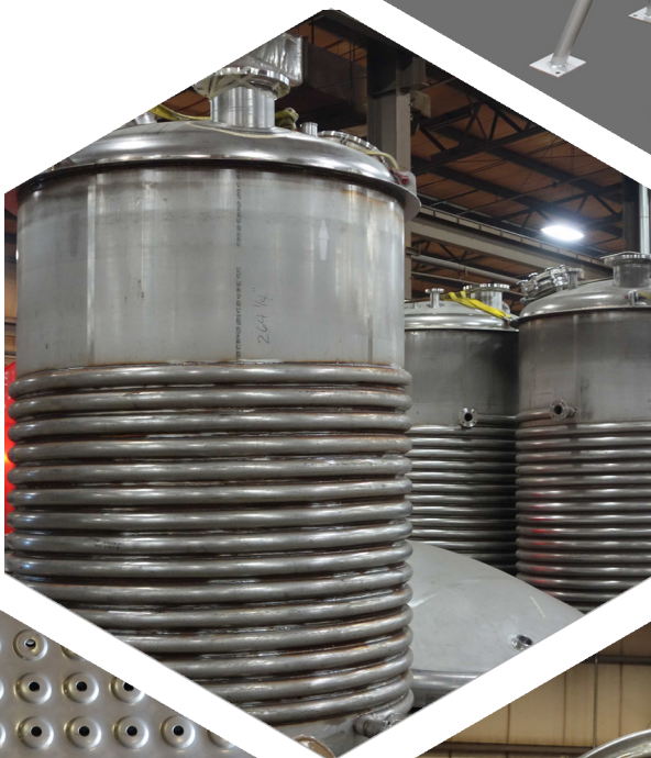
▶ Large ASME Vessels with half pipe jacket construction
